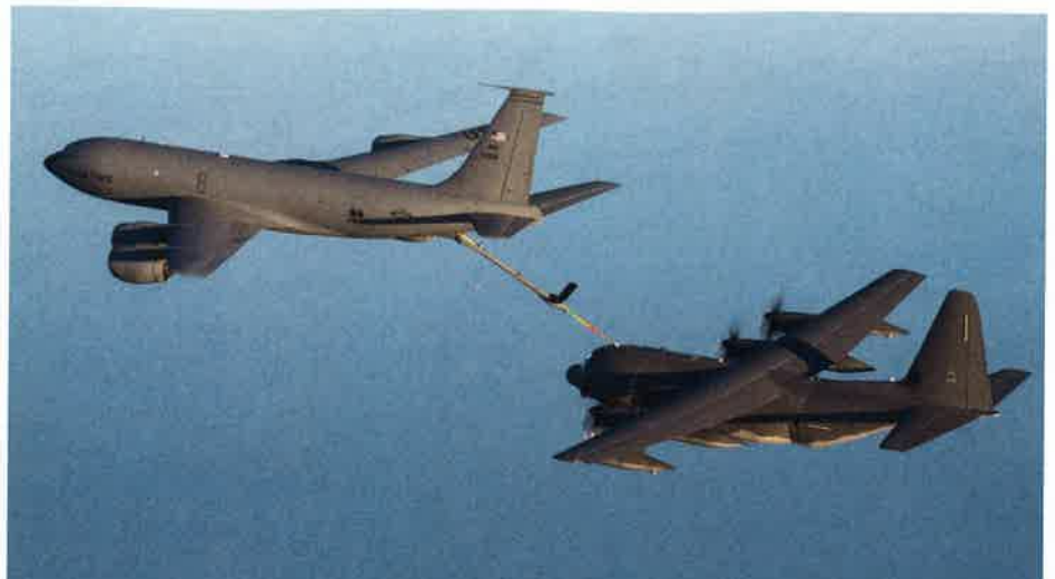
Above: In the US armed forces, only the C-130s of the AFSOC are capable of aerial refuelling. The aircraft are equipped with receptacles to 'take on gas' from boom-equipped tankers such as the KC-135R.
